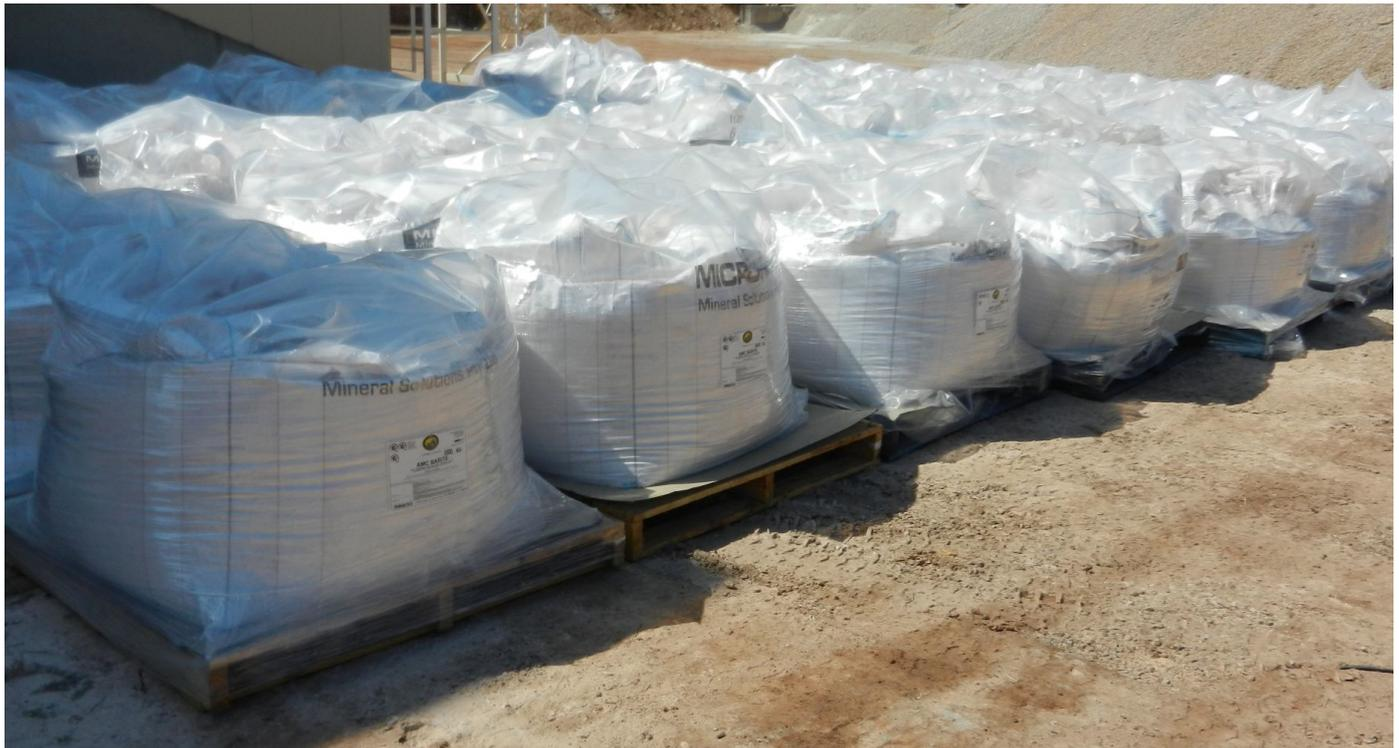
Barite is used by the petroleum industry as a weighting material in formulation of "drilling mud". Barite increases the hydrostatic pressure of the drilling mud allowing it to compensate for high-pressure zones experienced during drilling. The softness of the mineral also prevents it from damaging the drilling tools during the drilling process and enables it to serve as a lubricant.
